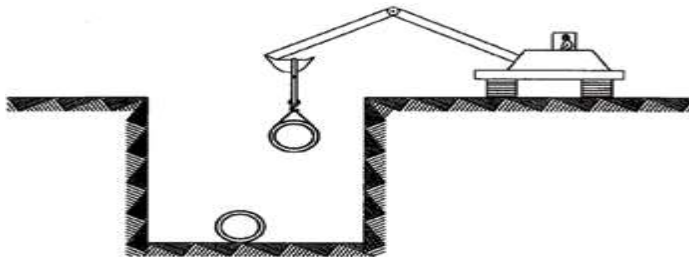
Fig 3: Mechanical lowering with excavator
